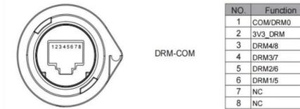
Step 2: Connect one end of the network cable to the corresponding port on the inverter.
