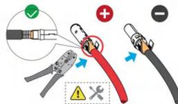
Step 3: Lead the cable through the cable gland and insert the crimp contact into the insulator until it audibly snaps into place. Pull the cable gently backward to ensure a firm connection. Tighten the cable gland and insulator using a torque of 2.5 N.m to 3 N.m.
